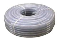
ATP Dura-Pure® NSF 61 ® PVC Hose is manufactured with a polyester spiraled yarn allowing the hose to be used in higher working pressure applications. It also complies with FDA regulations, and is Phthalate Free and NSF 61® certified for use in potable water and food beverage applications. It provides good chemical resistance, is lightweight, flexible and economically priced.
